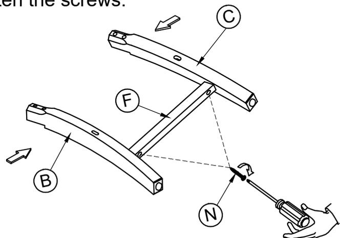
STEP 3: Do not fully tighten the bolts.
