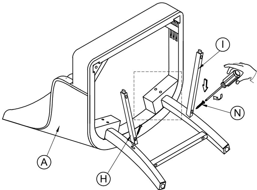
STEP 5: Do not fully tighten the screws.
