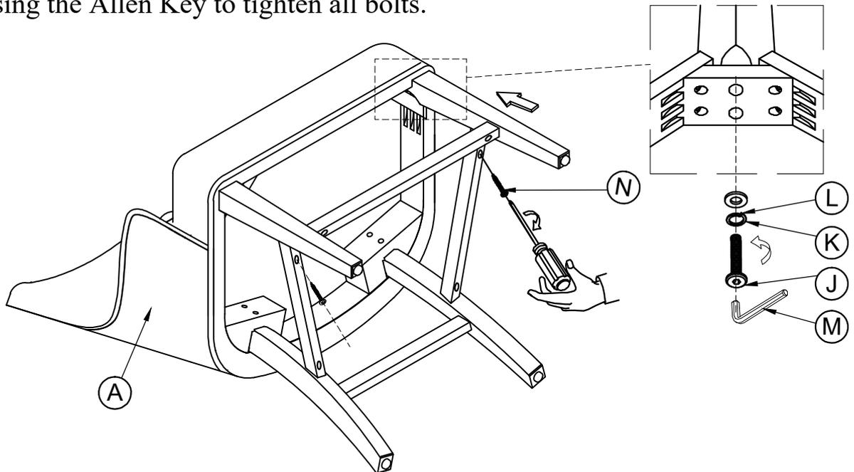
STEP 7: Using the Philips Head Screw driver to tighten all screws.
