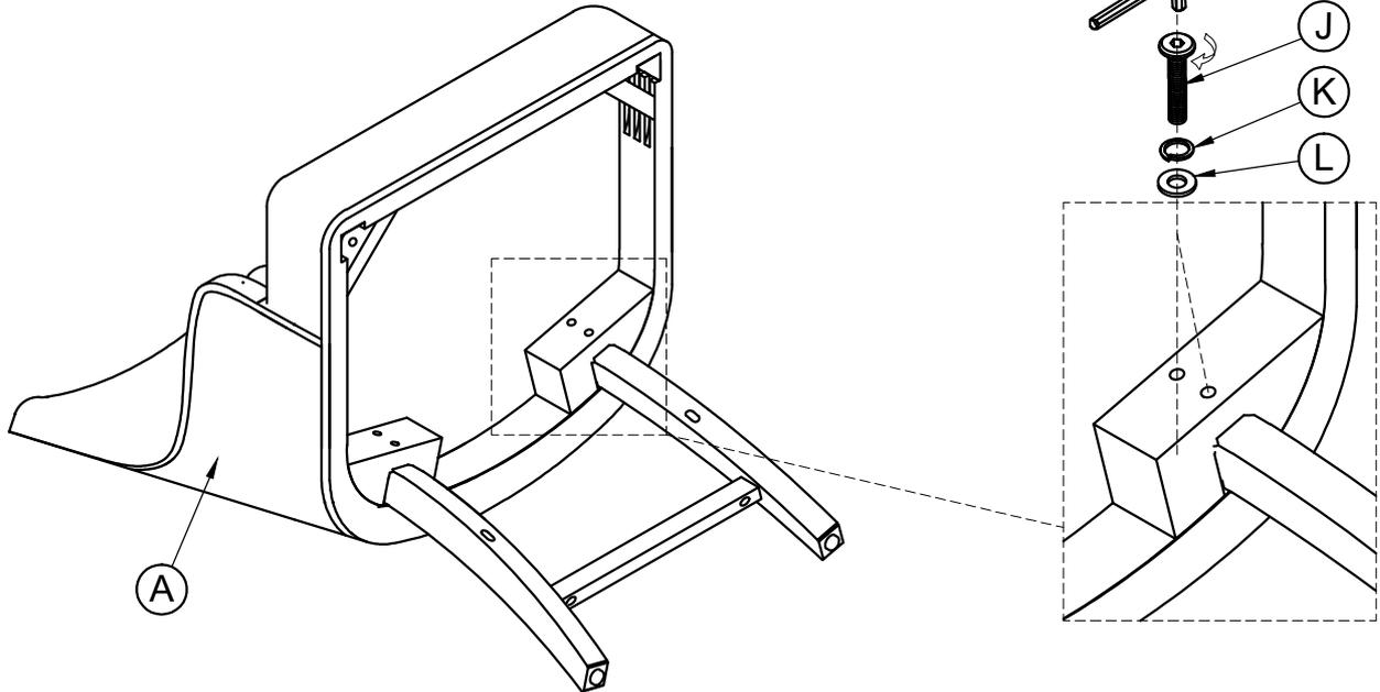
STEP 4: Do not fully tighten the screws.
